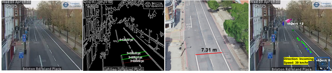
■ Figure 6 (L-R) a) TfL Camera Image at Brixton Road/Island Place, b) Edge Detection to Identify Lanes, c) Distance Identification Using Google Earth Referencing , d) Object Identification, Tracking, Direction and Speed Estimation
