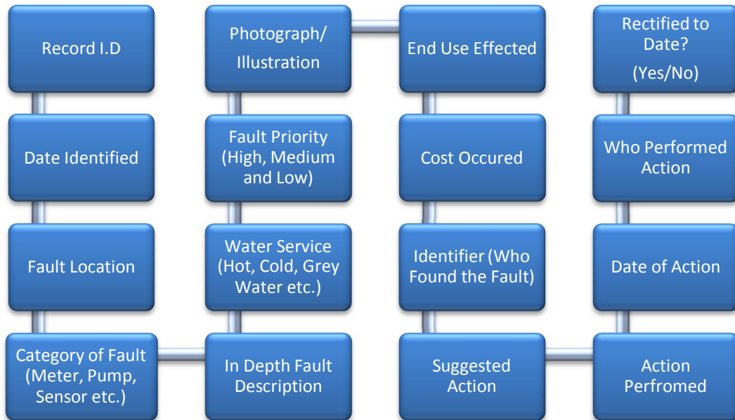
Figure 2. Suggested columns to be used when defining faults found in a building's water network.
