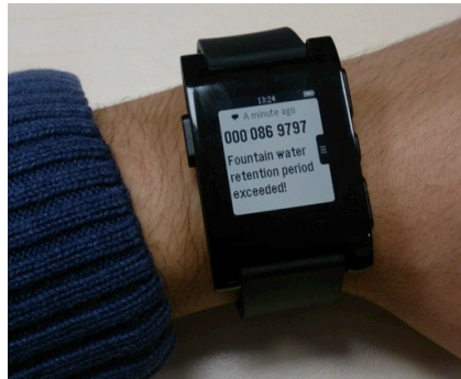
Fig. 8 Wearable info-centre, receiving notification from the water retention time observer
